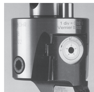
Adjusting Accuracy \varnothing 0.002 mm
