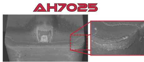
Tool wear after 60 grooves
