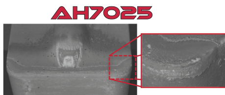
Tool wear after 60 grooves
